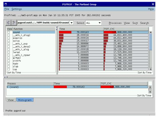
Figure 2-13: Profile with Hardware Event Counter
